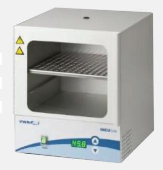
**Digital Controls:** The temperature can be freely adjusted in increments of 0.1°C up to a maximum of 70°C. Heating elements are incorporated into the housing base and walls to ensure temperature stability and uniformity.
